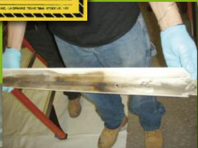
Samples of leaked PCBs hidden behind metal plate that covers lighting ballast found during EPA spot inspections.
